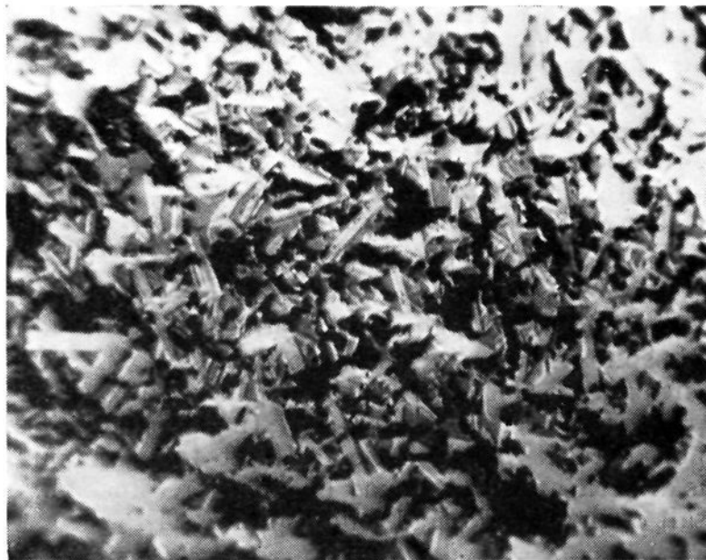
Fig. 2.—1500 \times unetched. Lightest, best defined phase is TiB_2 and the other is TiB_x . Black areas are voids.
